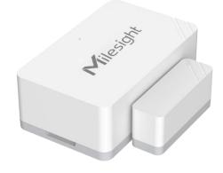
Milesight WS301 simply enables you to know when someone enters the office/building through door/window or something has been moved. The minimal magnet is placed inside the portable part, while the sensor is inside the fixed part that can be attached on door/window or other objects. With a style of minimalism and compact size, the wire-free WS301 can be easily mounted on the doors, panes, or cabinets, greatly providing real applications for smart homes, smart office or smart factories.
