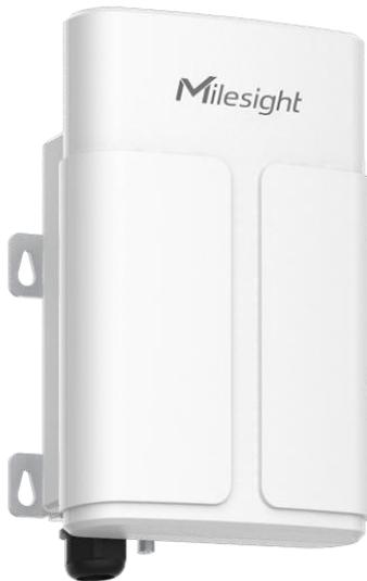
UG67 is a robust 8-channel outdoor LoRaWAN® hotspot, which is compatible with Helium LongFi technology. Adopting SX1302 LoRa chip, high-performance quad-core CPU and secure crypto chip, UG67 provides high-efficiency and reliable connection. UG67 has line of sight up to 15 km and can cover about 2 km in urbanized environment, which can cover larger areas with other hotspots.
