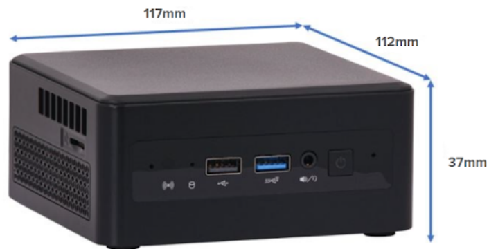
Figure 12: Moonstone “Slim Height” / Width / Length Dimensions
